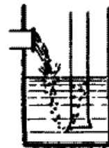
Fig. 6(b) Supply line should extend down into the sump to prevent the churning of air into the water.
